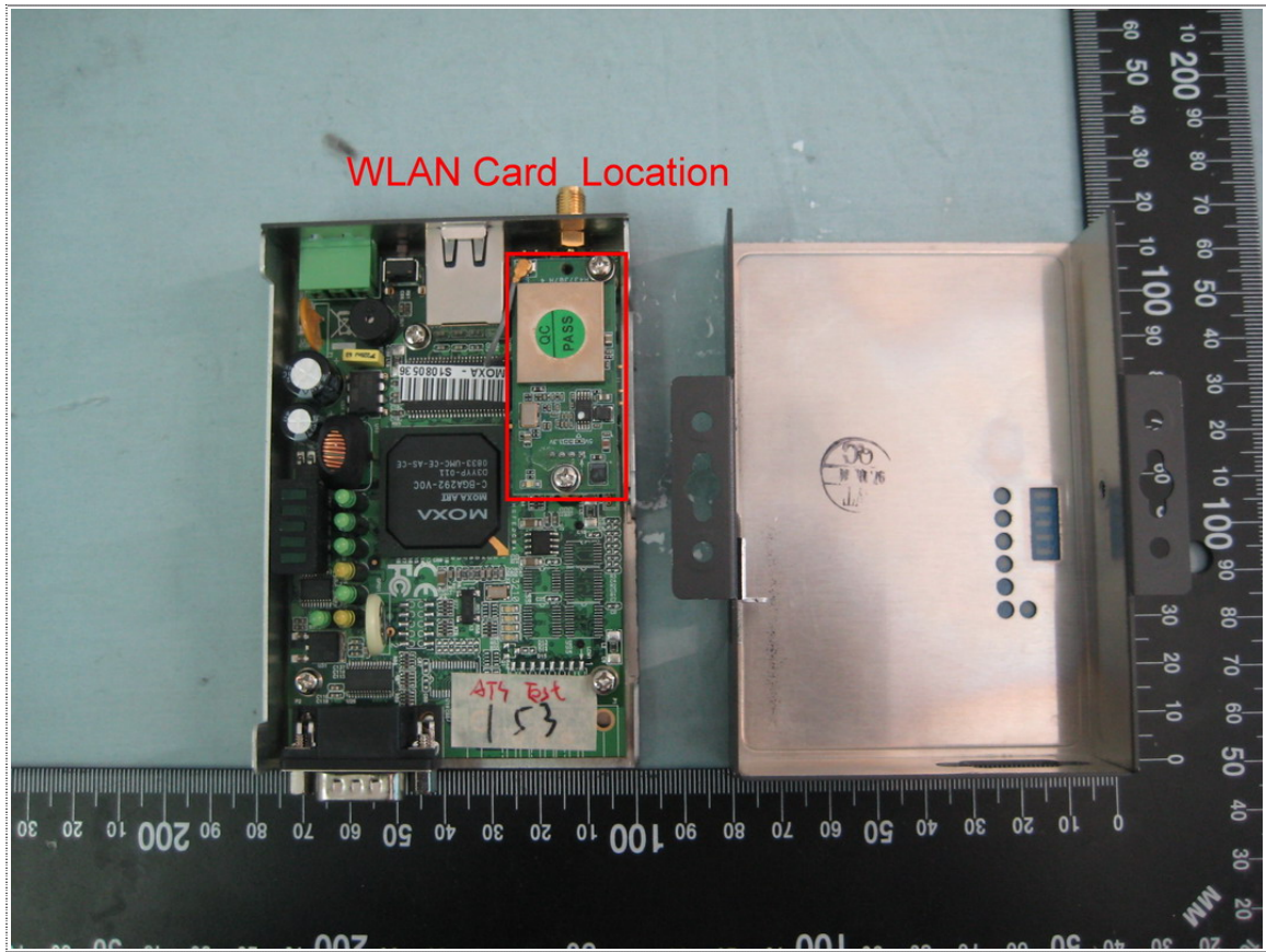
WLAN module Location
