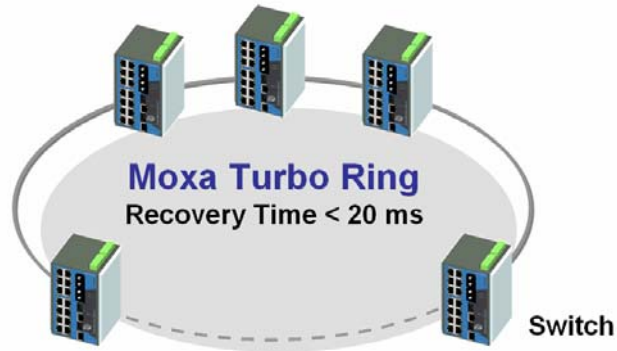
Figure 3: Example of ring redundancy
