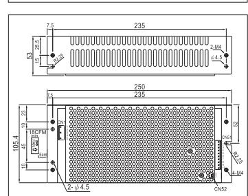
AC input voltage range .....90~264VAC; 127~370VDC
