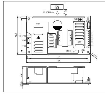
AC input voltage range ..... 90~264VAC; 127~370VDC
