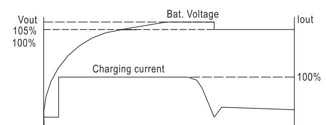
Type B: 2 section voltage charger (detect on charging current)
