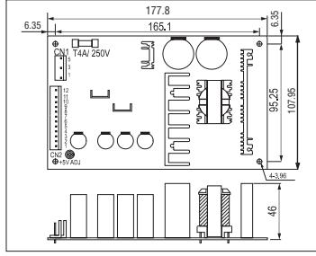
AC input voltage range ..90~264VAC; 127~370VDC
