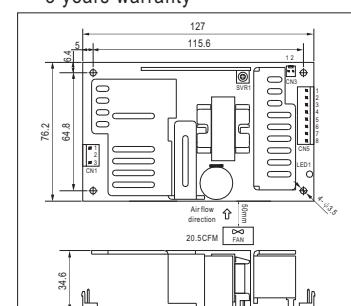
AC input voltage range .....90~264VAC; 127~370VDC
