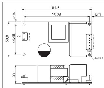
AC input voltage range .....90~264VAC; 127~370VDC
