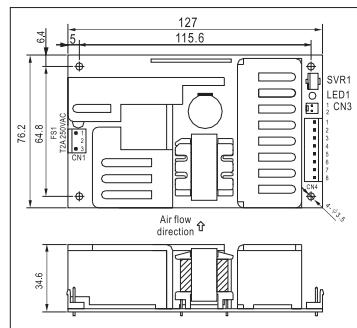
AC input voltage range ..... 90~264VAC; 127~370VDC
