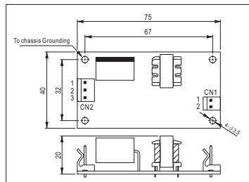
AC input voltage range ..... 85~264VAC; 120~370VDC
