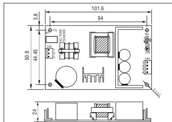
AC input voltage range ..... 90~264VAC; 127~370VDC
