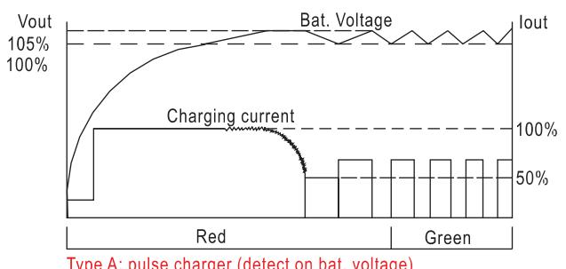
Type A: pulse charger (detect on bat. voltage)
