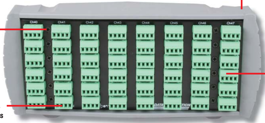
Figure 4. Every channel provides direct RTD or precision voltage connections as shown above.
