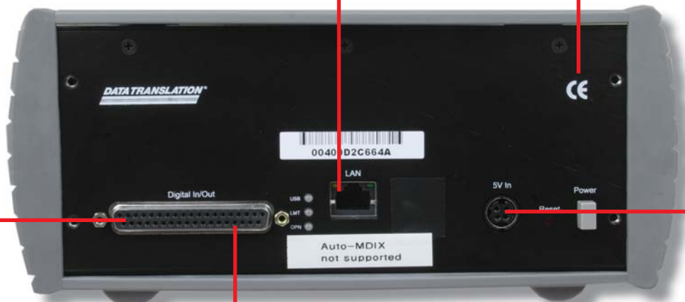
Figure 5. Digital I/O, power, and USB or Ethernet connections are provided on the back panel.
