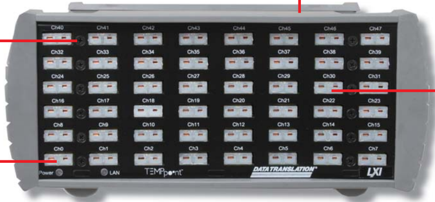
Figure 3. Every channel provides direct thermocouple or precision voltage connections as shown above.
