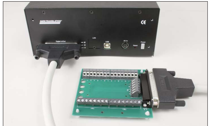
Figure 6. Digital inputs and outputs are easily connected via the 37-pin D-sub connector on the back of the instrument using the STP-37 screw terminal panel and 37-pin EP333 cable.
