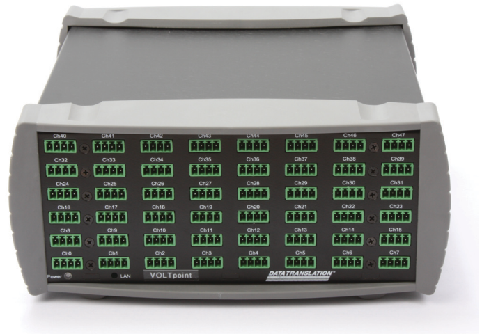
Figure 1. VOLTpoint allows direct battery cell connection of voltages up to \pm 400V with 1000V isolation between any of the 48 channels. Ground loops are eliminated through the isolation of each channel using the ISO-Channel technology. The \pm 10V range allows resolution and accuracy of less than 300 microvolts. The \pm 400V range is available for measuring stacked cells or higher voltages.
