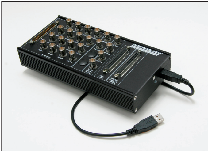
Figure 9. The DT9818 is also available in a BNC boxed version that houses the DT9818-OEM board. This model is useful for OEM prototypes and end-user applications. Models are: DT9818-16SE-BNC for a single-ended analog input configuration, and the DT9818-8DI-BNC for differential inputs.
