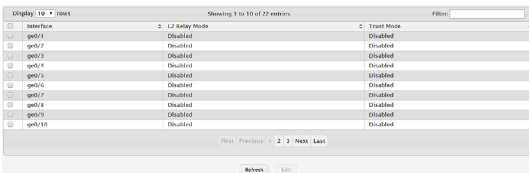
Figure 4.185 Switching > DHCP Snooping > L2 Relay > Interface Configuration
