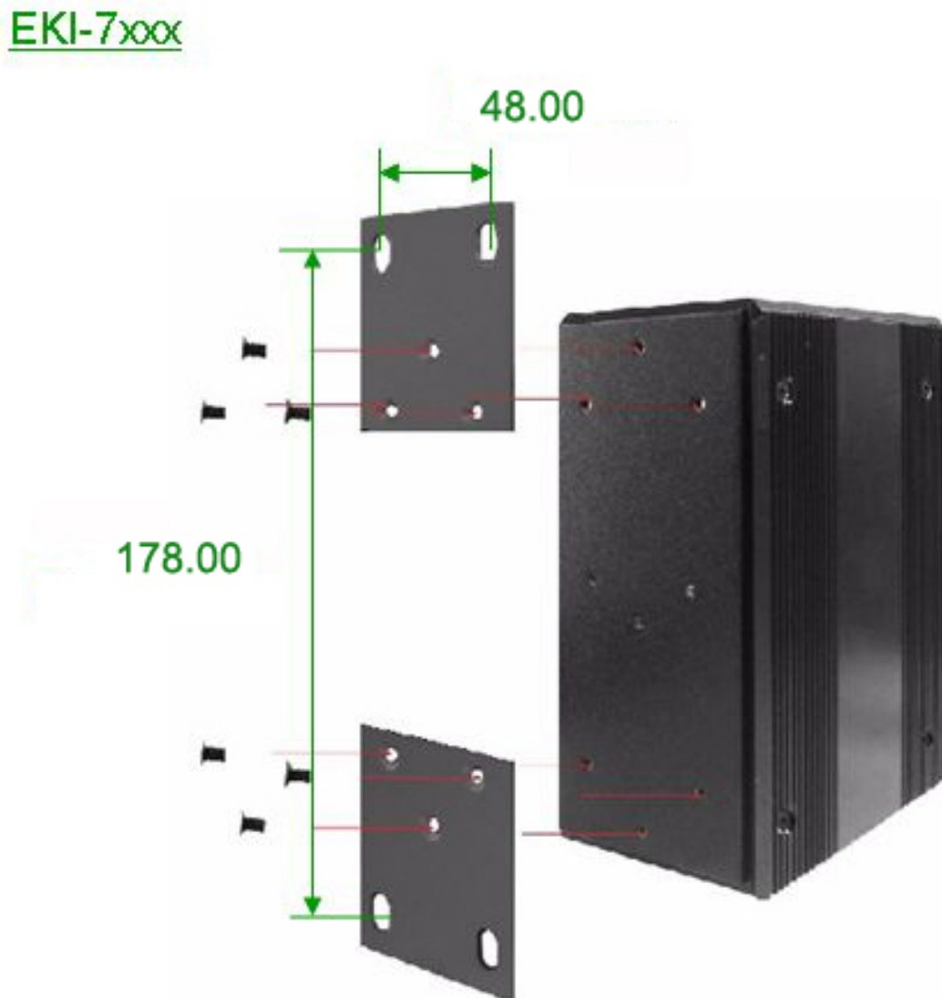
Figure 2.5: Combine the Metal Mounting Kit (units: mm)
