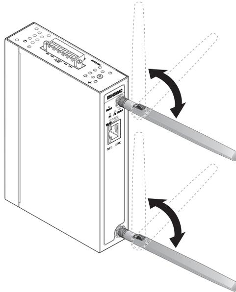
**Figure 2.11 Positioning the Antenna**
