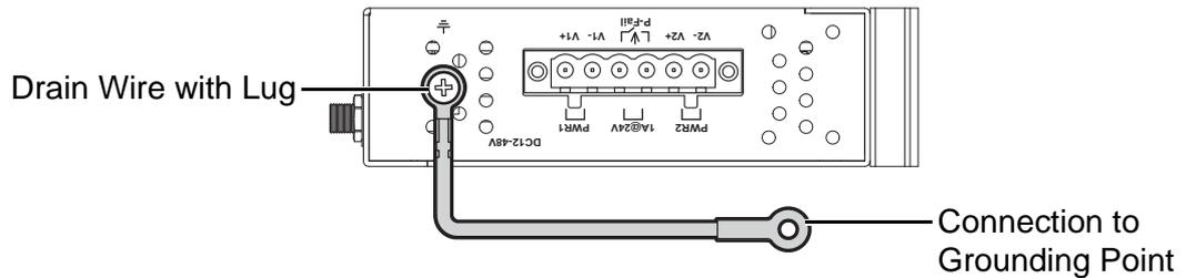
**Figure 2.14 Grounding Connection**
