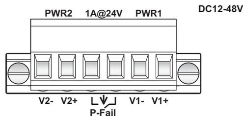
**Figure 2.16 Terminal Receptor: Power Input Contacts**
