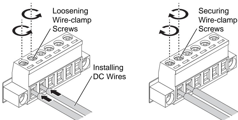
**Figure 2.18 Installing DC Wires in a Terminal Block**
