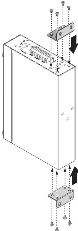
**Figure 2.8 Installing Wall Mount Plates**
