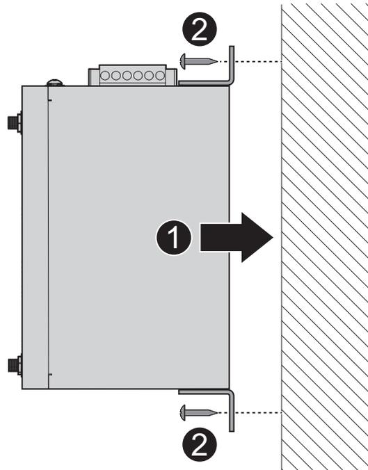
**Figure 2.9 Wall Mount Installation**
