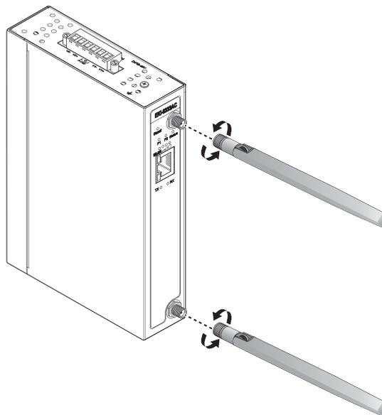
**Figure 2.10 Installing the Antenna**
