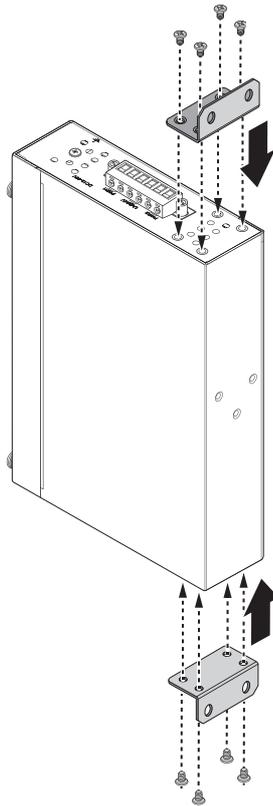
**Figure 2.8 Installing Wall Mount Plates**
