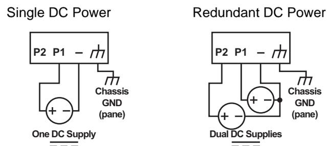
Figure 2.13 Power Wiring for EKI-6333AC-A Series
