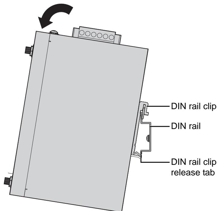
Figure 2.5 Installing the DIN Rail Kit
