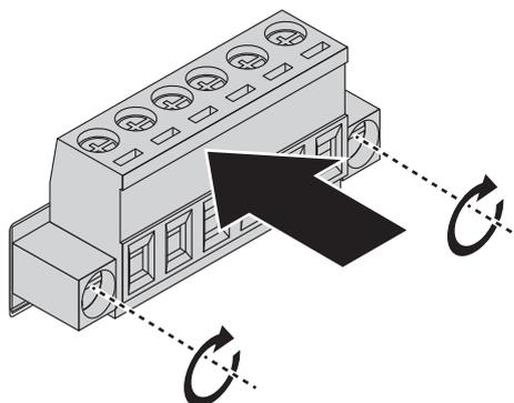
**Figure 2.19 Securing a Terminal Block to a Receptor**
