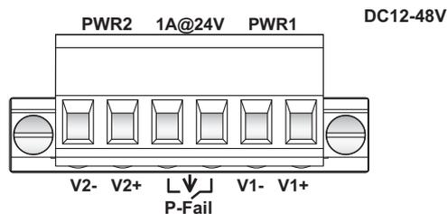
**Figure 2.15 Terminal Receptor: Relay Contact**
