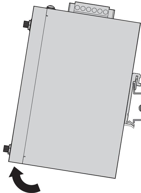
**Figure 2.7 Removing the DIN Rail**
