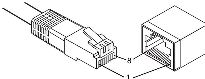
**Figure 2.12 Ethernet Plug & Connector Pin Position**
