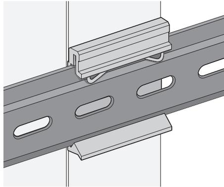
**Figure 2.6 Correctly Installed DIN Rail Kit**
