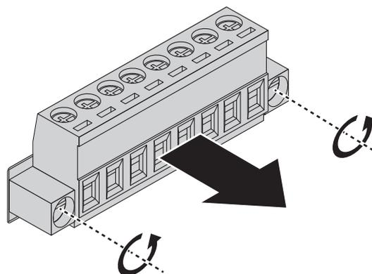
**Figure 2.19 Removing a Terminal Block**
