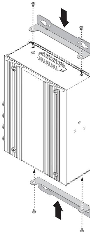
**Figure 2.8 Installing Wall Mount Plates**
