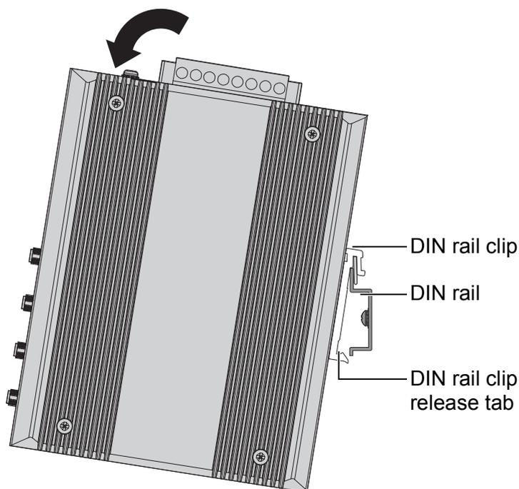
Figure 2.5 Installing the DIN Rail Kit
