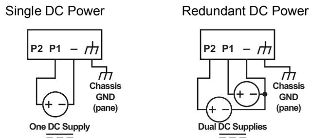
**Figure 2.15** Power Wiring for EKI-6333AC-4GP
