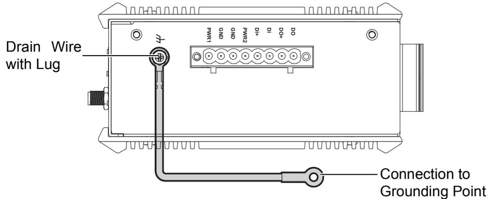
**Figure 2.16 Grounding Connection**
