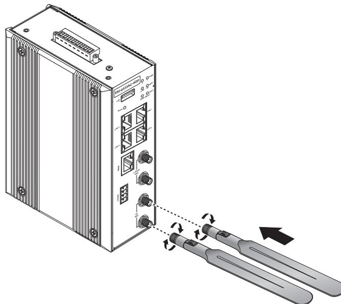
**Figure 2.10 Installing the Antenna**
