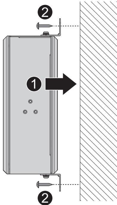
**Figure 2.9 Wall Mount Installation**
