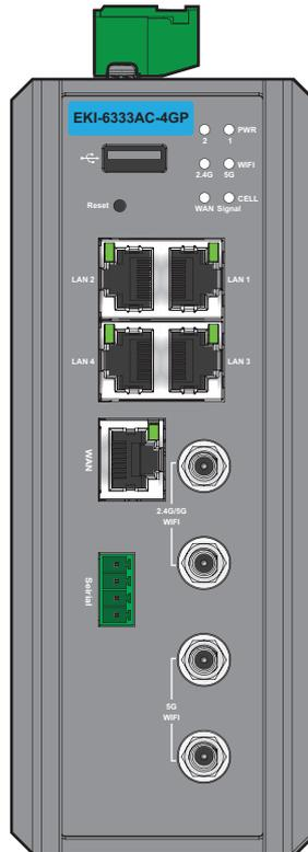
Figure 2.4 System LED Panel
