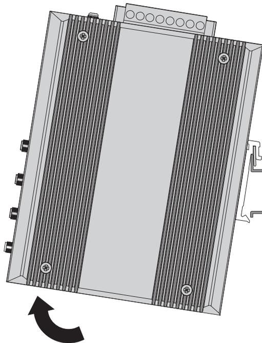
**Figure 2.7 Removing the DIN Rail**
