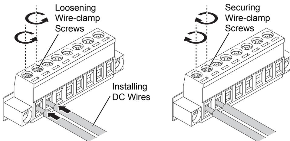
**Figure 2.20 Installing DC Wires in a Terminal Block**
