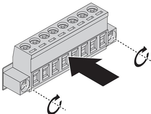
**Figure 2.21 Securing a Terminal Block to a Receptor**
