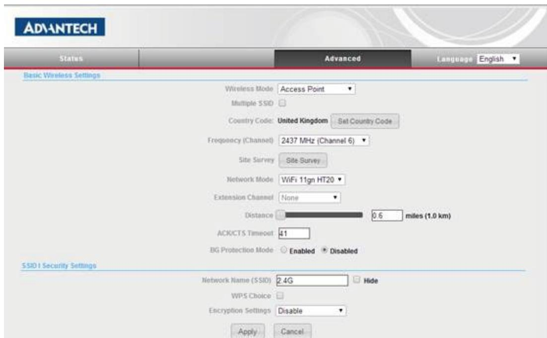
**Figure 3.7 Basic Wireless Access Point Settings**
