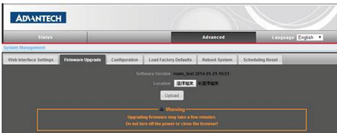
Figure 7.3 Firmware Upgrade Setting
