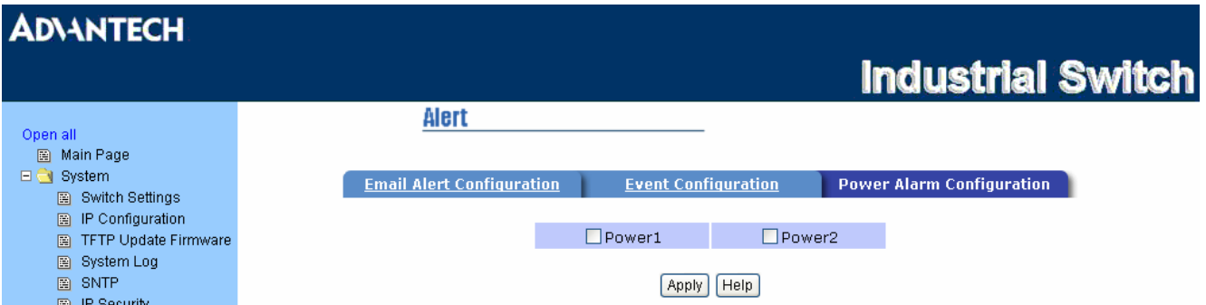
Figure 3.14: Power Alarm Configuration
