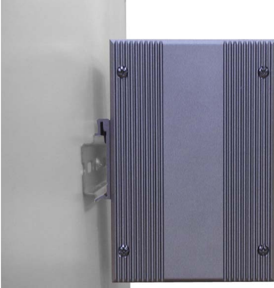
Figure 2.5-3 Installation to DIN-rail Step 2
