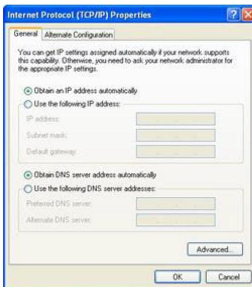
Click “OK”, EKI-1334 will allocate an IP address: 192.168.2.x, and a gateway: 192.168.2.1(the default address of EKI-1334).
