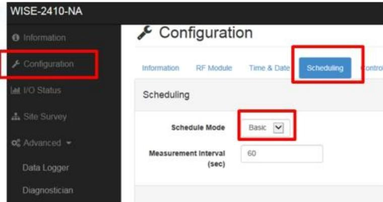
Scenario B: Sensing target on specific timing for better power saving application. In this example: Mon. 8:00am ~ Sun. 8:00 am.
