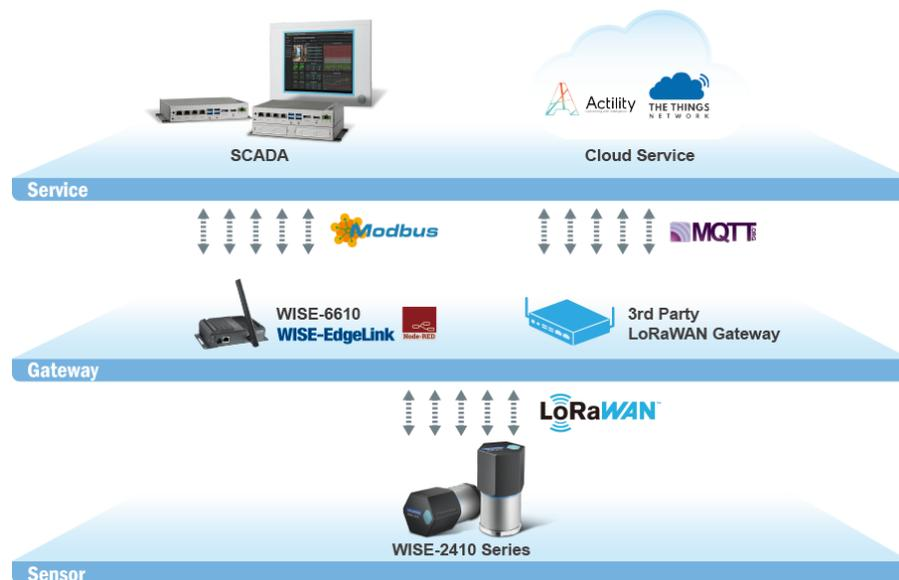
Figure 1.1 System Architecture
