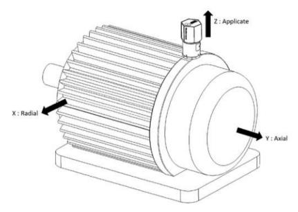
Figure 3.3 WISE-2410X Installation Direction on motor
