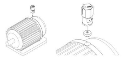
Figure 3.8 Adhesive Mounting Pad
