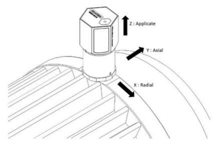
Figure 3.4 WISE-2410X Detail Installation Direction on motor
