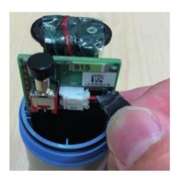
Figure 3.10 Battery Replacement Step 2
