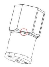
Figure 3.2 Tighten two chassis
