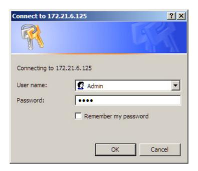
Once logged in, the user <u>must</u> change the device name. The device name box may have a sample such as APAX-5520. A suggestion is to change the name to "APAX-5520-1". Other controllers on the same network can have subsequent numbers or different names but all controller names on the same network must be unique.
