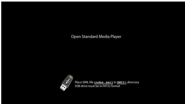
After performing the initial setup as outlined above, the player will boot into the "Open Standard Media Player" screen. Plug in a USB keyboard to enter configuration menus.
