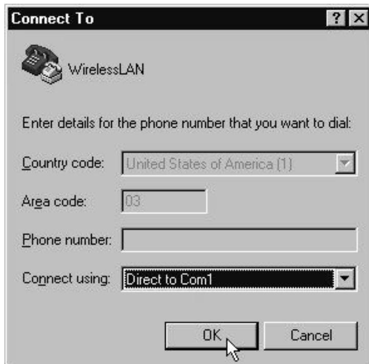
5. Set the port settings to **57600 bps, 8 data bits, no parity, no flow control**. Click **OK**.
