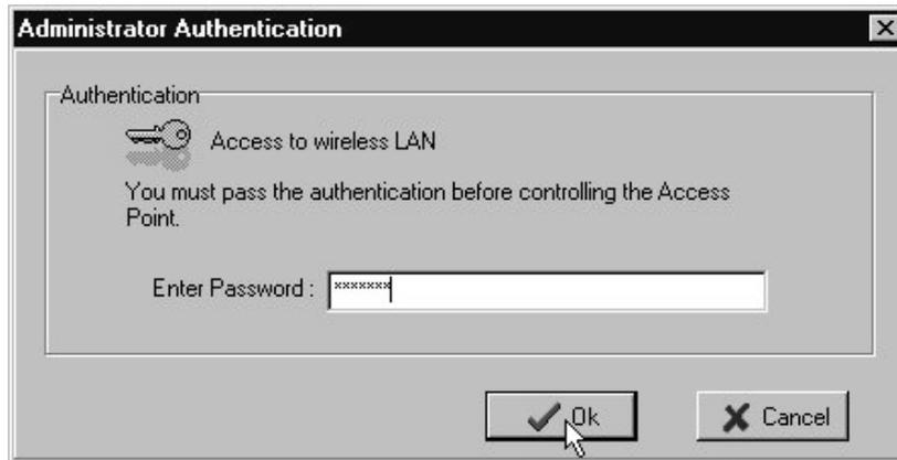
7. After entering the correct password, a configuration window appears. You will see the basic information of the Access Point, such as MAC Address, Frequency Domain and Firmware Version.
