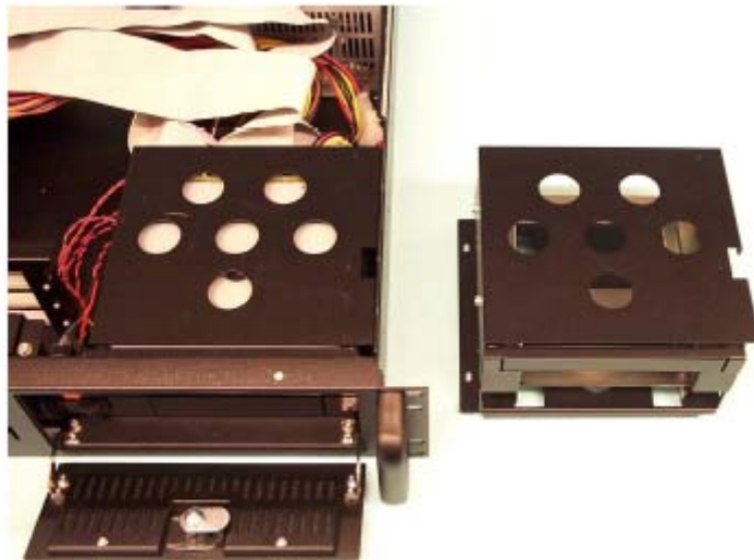
Fig 2-9 Drive Bay Installation
