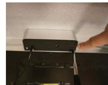
Fasten the 2 screws to fix the peripheral in place
