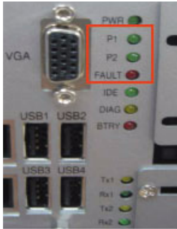
Figure 2.12: LED Locations to Monitor Power Input
