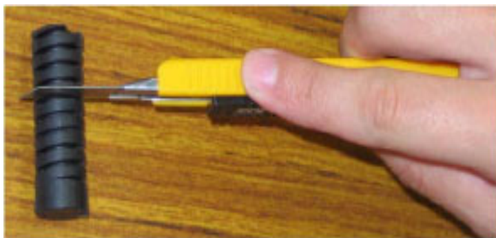
Figure 3.3: Adjust the Anti-Vibration Rubber
