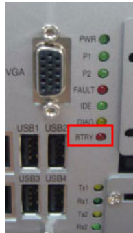
Figure 2.14: LED Location for Battery Backup
