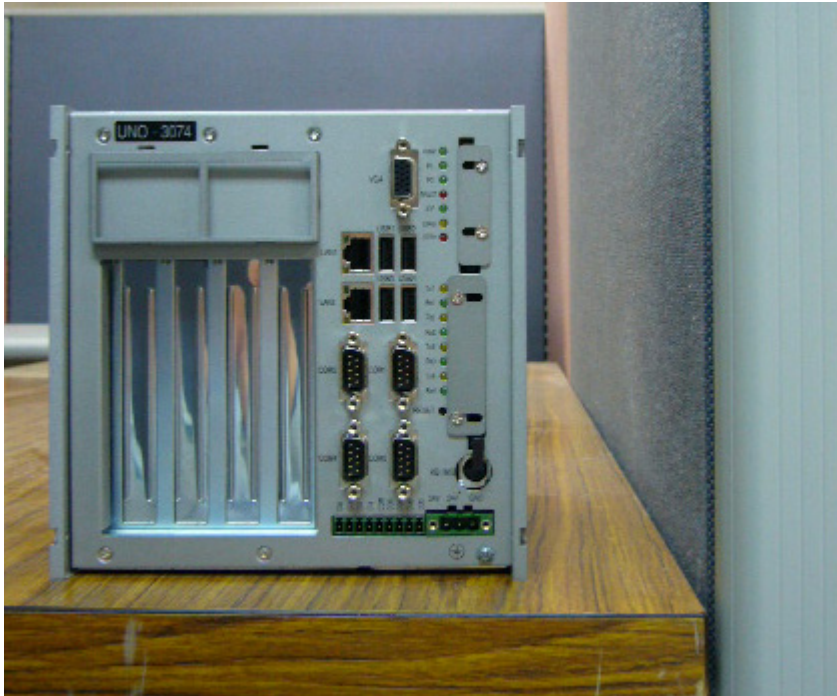
Figure 3.7: UNO-3074 Correct Installation
