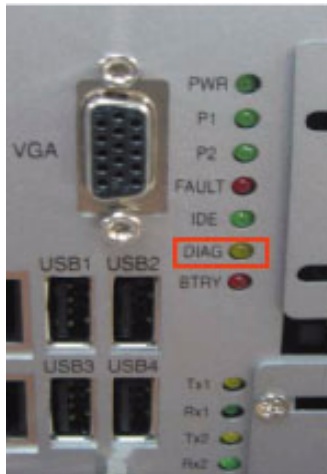
Figure 2.13: LED Location for System Diagnosis
