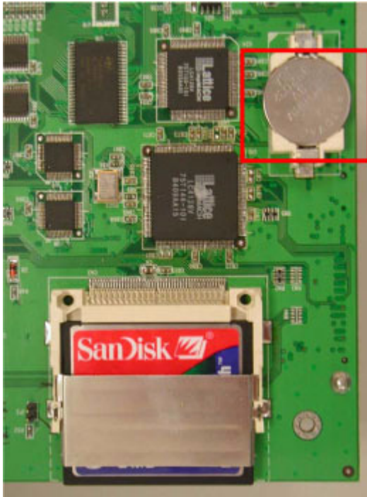
Figure 2.15: Lithium Battery for SRAM
