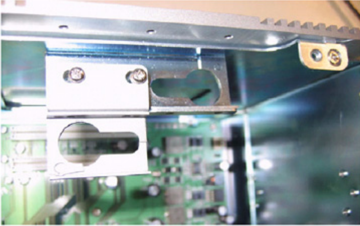
Figure 3.2: 2nd PCI-bus Card Installation
