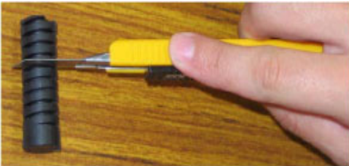
Figure 3.3: Adjust the Anti-Vibration Rubber
