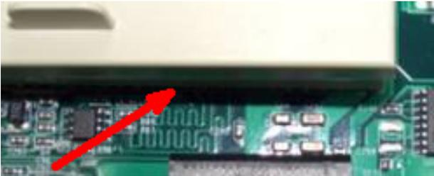
5. Plug-in PCI-bus card in a PCI-slot of UNO-3072LA.
