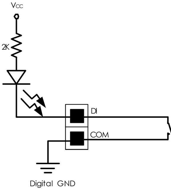
**Figure 2.5: Isolated Digital Input Connection- Dry Contact**
