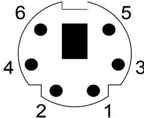
**Table A.7: Keyboard and Mouse Connector Pin Assignments**
