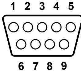
**Table A.2: RS-232 Standard Serial Port Pin Assignments**
