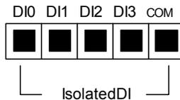
*Figure 2.3: Pin Assignment of Digital Input Connector*
