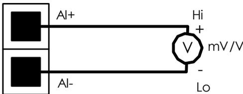
*Figure 2.9: Milli Volt and Volt Input*
