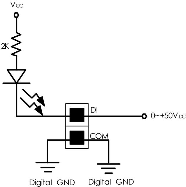
**Figure 2.4: Isolated Digital Input Connection- Wet Contact**
