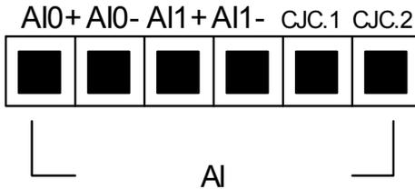
*Figure 2.8: Analog Input Connector Pin Assignment*
