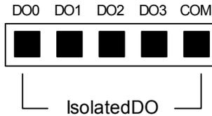
**Figure 2.6: Pin Assignment of Isolated Digital Output Connector**
