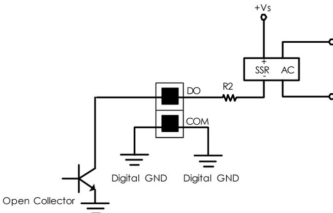
**Figure 2.7: Isolated Digital Output Connection**
