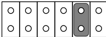
Enable Termination Resistor for CAN2 Port
