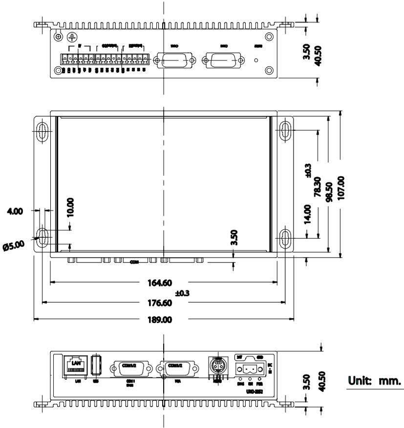
Figure 1.1: Chassis Dimensions
