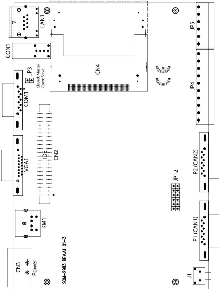
Figure A.1: UNO-2052 Connector and Jumper Location (Top View)
