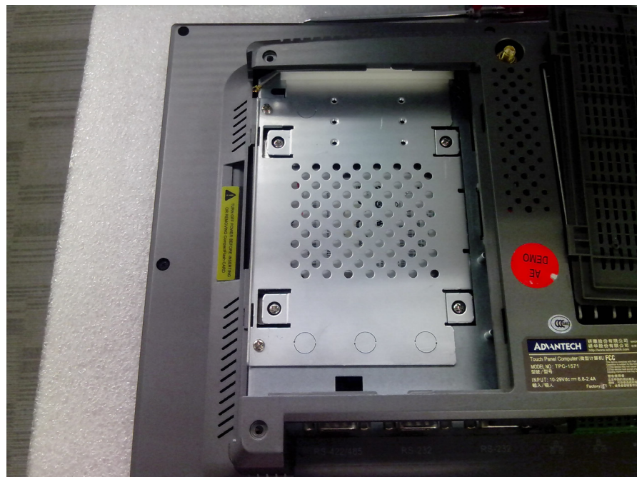
Figure C.2 Removing HDD bracket
