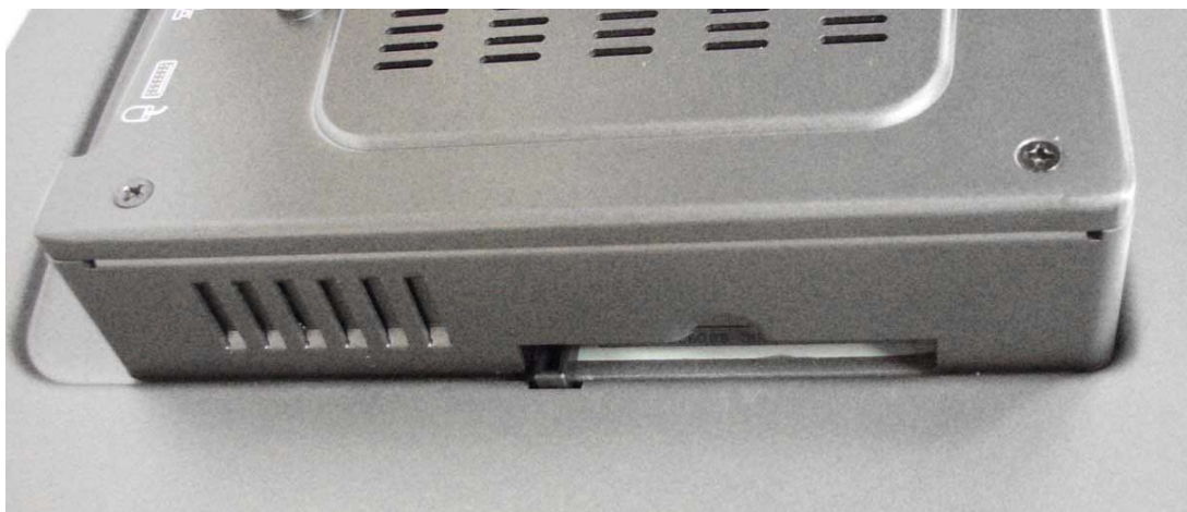
Figure 2.2 Install CompactFlash Memory Card
