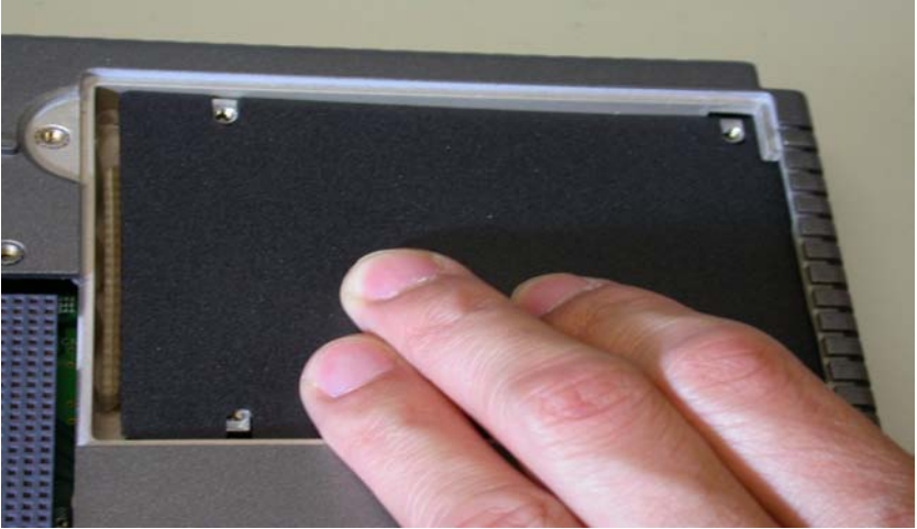
Figure E.19: Laying in the HDD insulator
