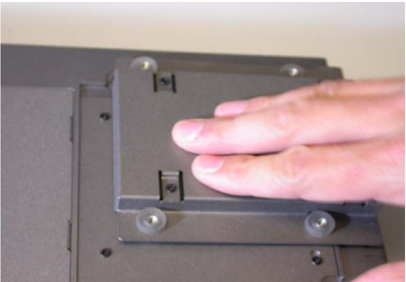
Figure E.12: Placing the HDD holder - 2
