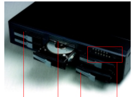
CD-ROM FDD Six hot-swappable Ultra 160 SCSI HDDs LEDs for power, fan, temperature, voltage, HDDs and LANs
