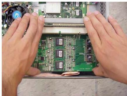
Plug the add-on card horizontally into PCI slot.
