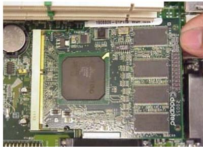
Insert the zero-channel hardware RAID module into RAID module socket with 30-degree angle.
