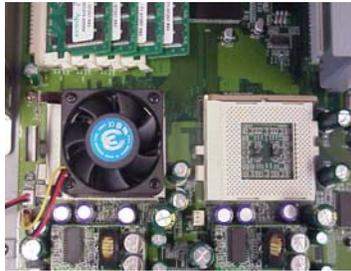
CPU Cooler Fan installed. Please repeat the same procedure to install another CPU and CPU cooler fan.
