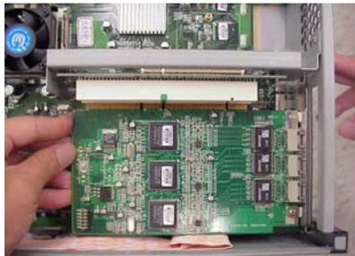
Remove the pre-installed bracket so that add-on card bracket can be inserted. Put down the add-on card.
