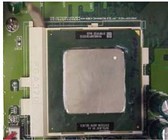
Orient the CPU to the socket correctly so that the pins match the receptacles. Insert the CPU in the socket so that the pins fully insert.
