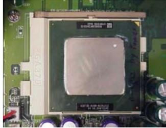
Lower the retaining lever so that the CPU locks in place and latch the arm to the side of the socket.
