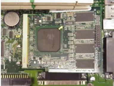
Please press the module down and let the bracket of module socket latch it.
