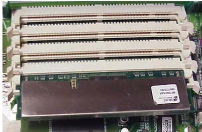
Press the module into the socket so that it seats firmly in place and the retaining latches rotate upwards and seat themselves in the notches on the side of the module.
