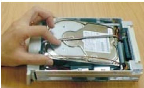
**Figure 1-7: Installing the Hard Disk Drive**
