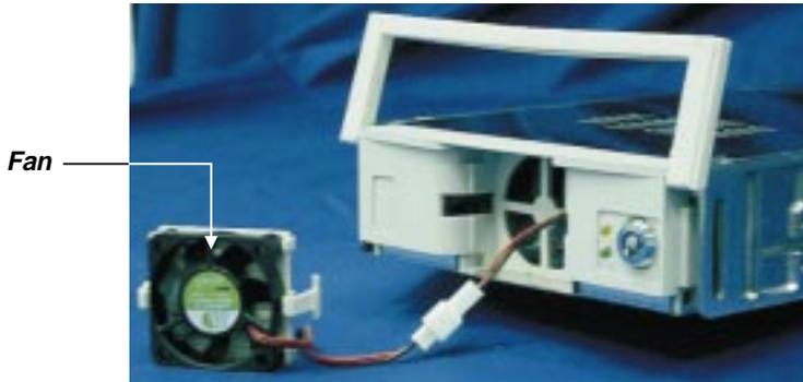
***Figure 3-6: Location of the Fan on the Fan Holder***
