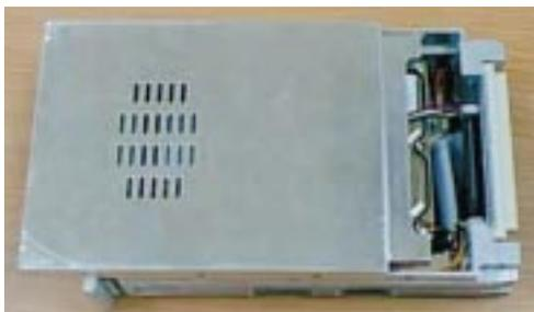
**Figure 1-5: Opening the Mobile Rack**
