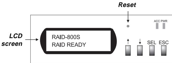
*Figure 1-2: Front View of the Controller*
