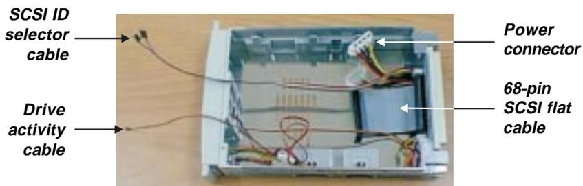
**Figure 1-6: Internal Structure of the Mobile Rack**
