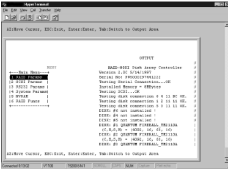
Figure 6-2: Configuring through a terminal
