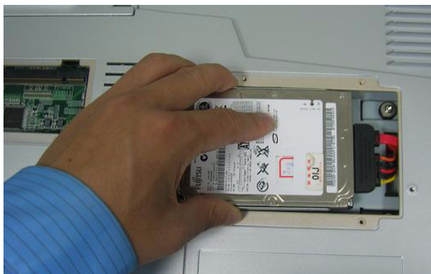
Figure 3.2 Connect the HDD to the HDD cable
