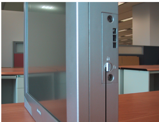
Power switch (Open status)
