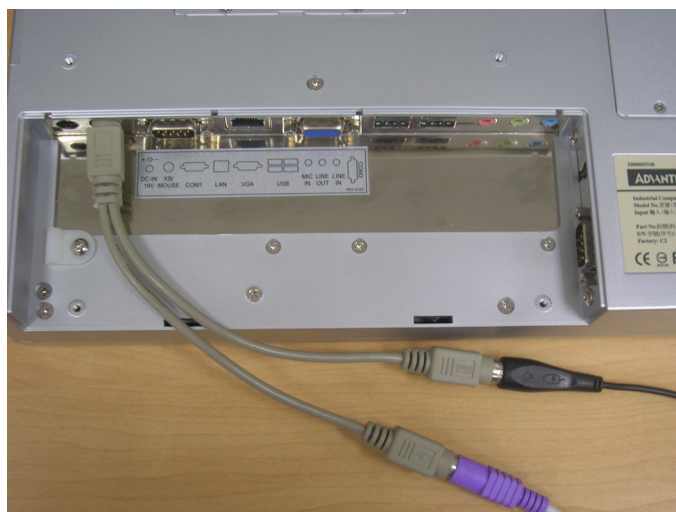
Figure 2.6 Connecting the Y-shaped adaptor to the PS2 mouse and keyboard
