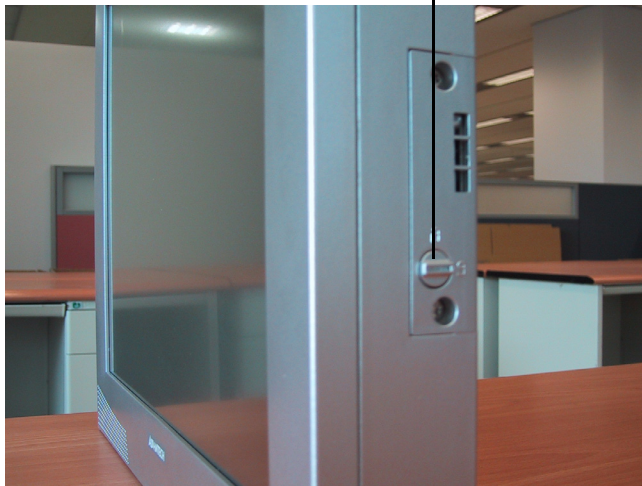
Figure 2.7 Power switch in lock status
