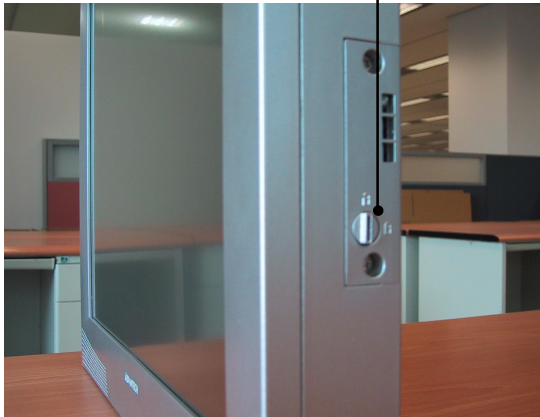
Figure 2-7: Power switch in open status
