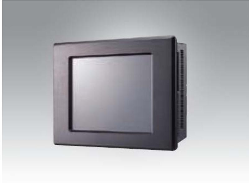
**Figure 2.1 Front View of the PPC-L61T Panel PC**
