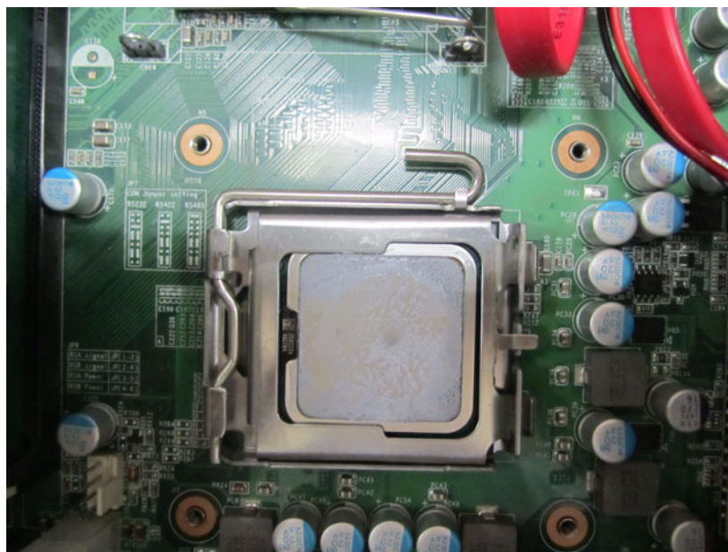
Figure 4.9 Fix CPU in the socket
