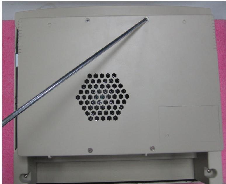
Figure 4.1 Unfastening the Rear Cover
