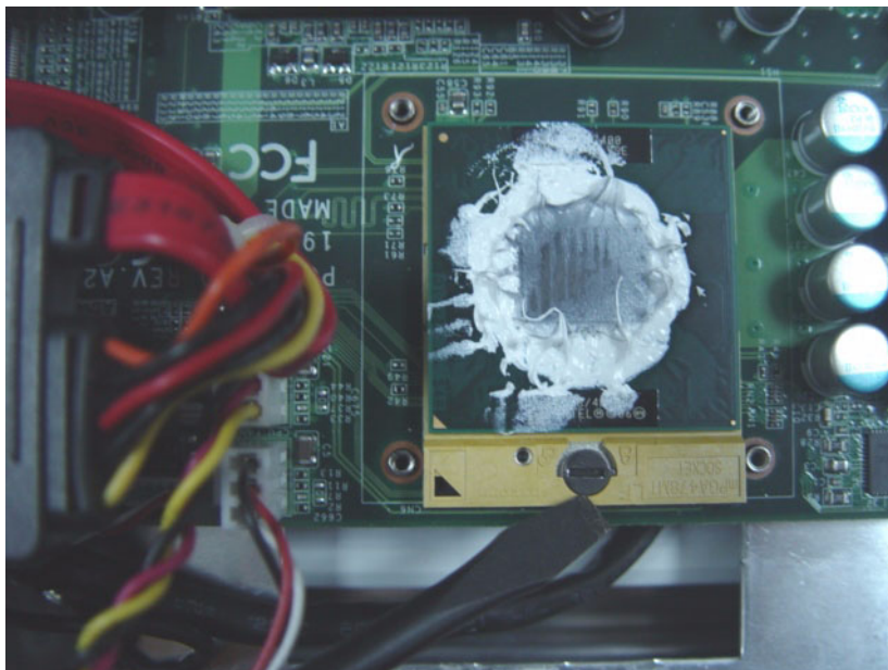
Figure 4.9 Tightening the Screws on the CPU
