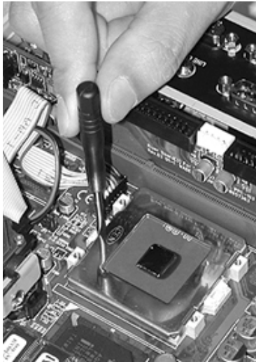
Figure 2-4: Insert screw driver into the hole
