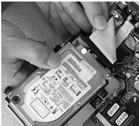
Figure 2-9: Connect flat cable to the HDD
