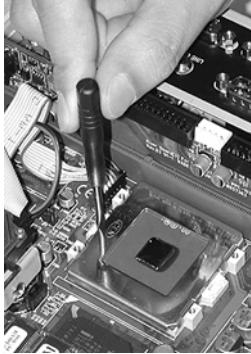
Figure 2.4: Insert screw driver into the hole
