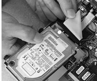
Figure 2.9: Connect flat cable to the HDD
