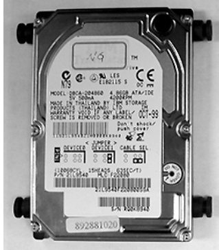
Figure 2.8: Rubber screwed onto the hard disk
