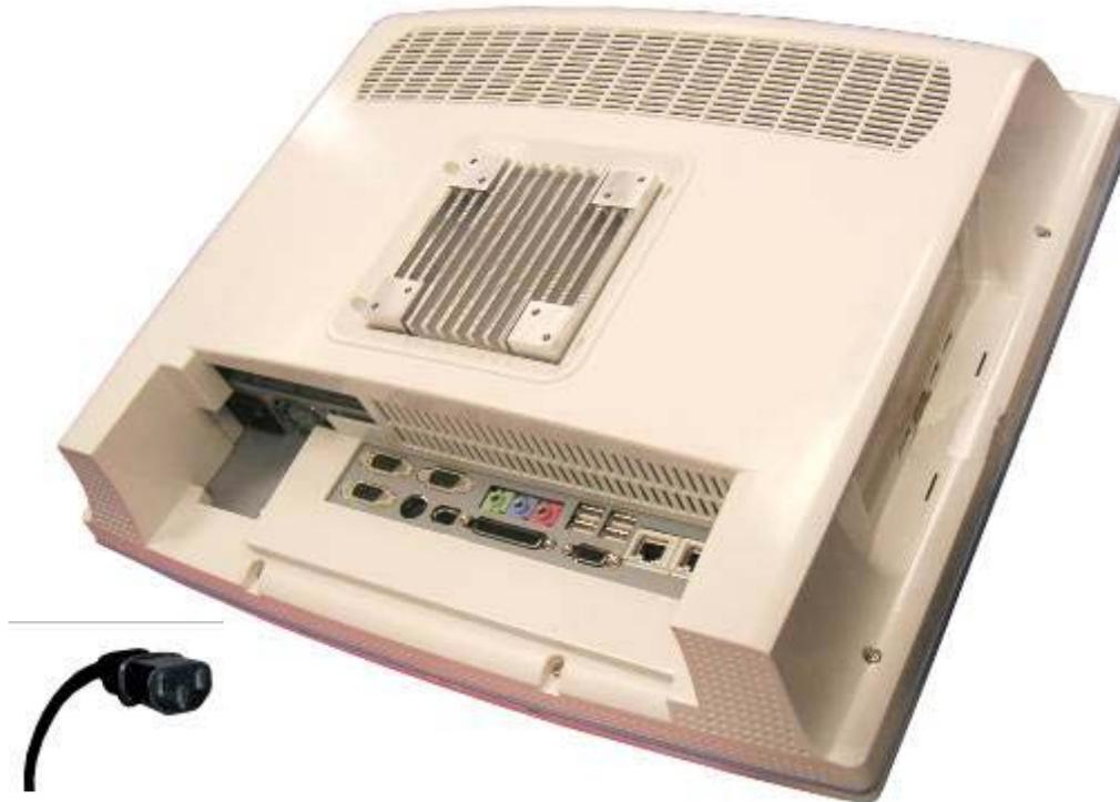
Figure 2-5: Connecting the power cord
