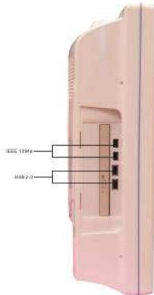
*Figure 2-2: Left side view of the Point of Care Terminal*
