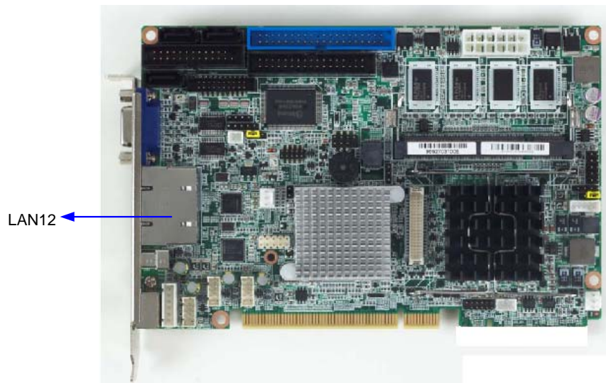
Figure 2.11 Dual Giga LAN RJ45 connector (LAN12)
