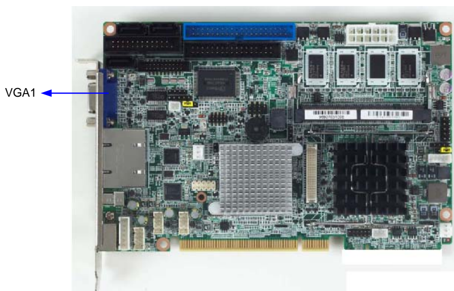
Figure 2.4 VGA Connector (VGA1)
