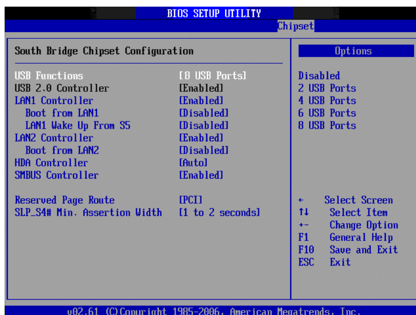
Figure 3.13 South Bridge Configuration
