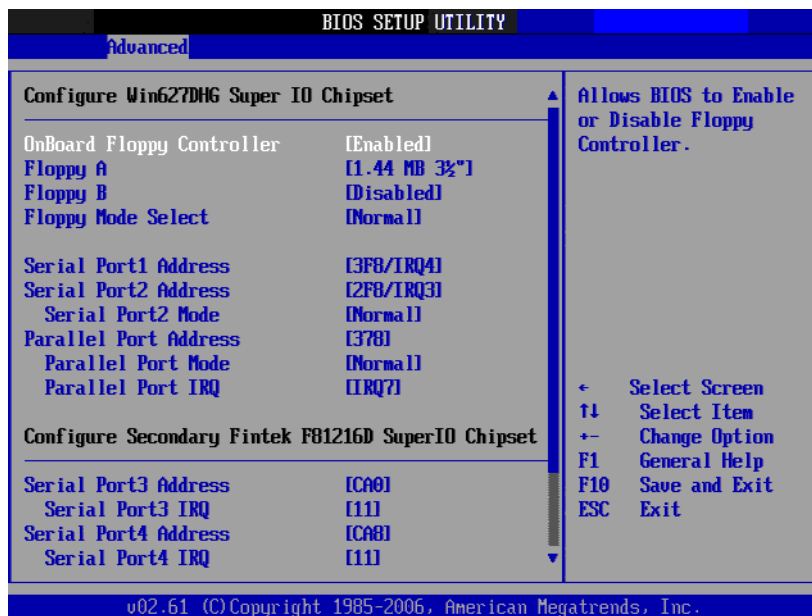
Figure 3.6 Super I/O Configuration
