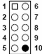
**Table B.18: Front Panel LAN Indicator connector (CN65)**
