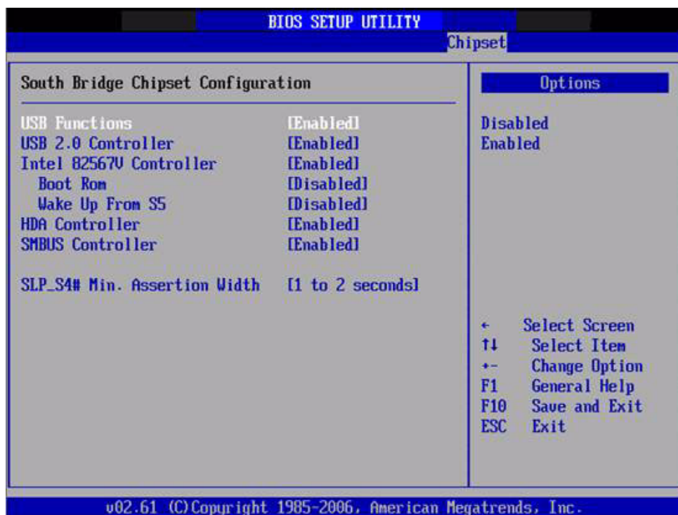
Figure 3.26 South Bridge Configuration
