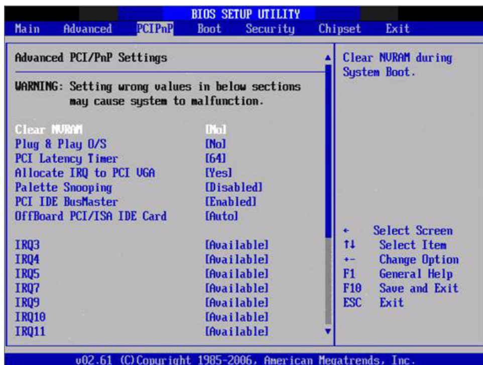
Figure 3.19 PCI/PnP Setup (top)
