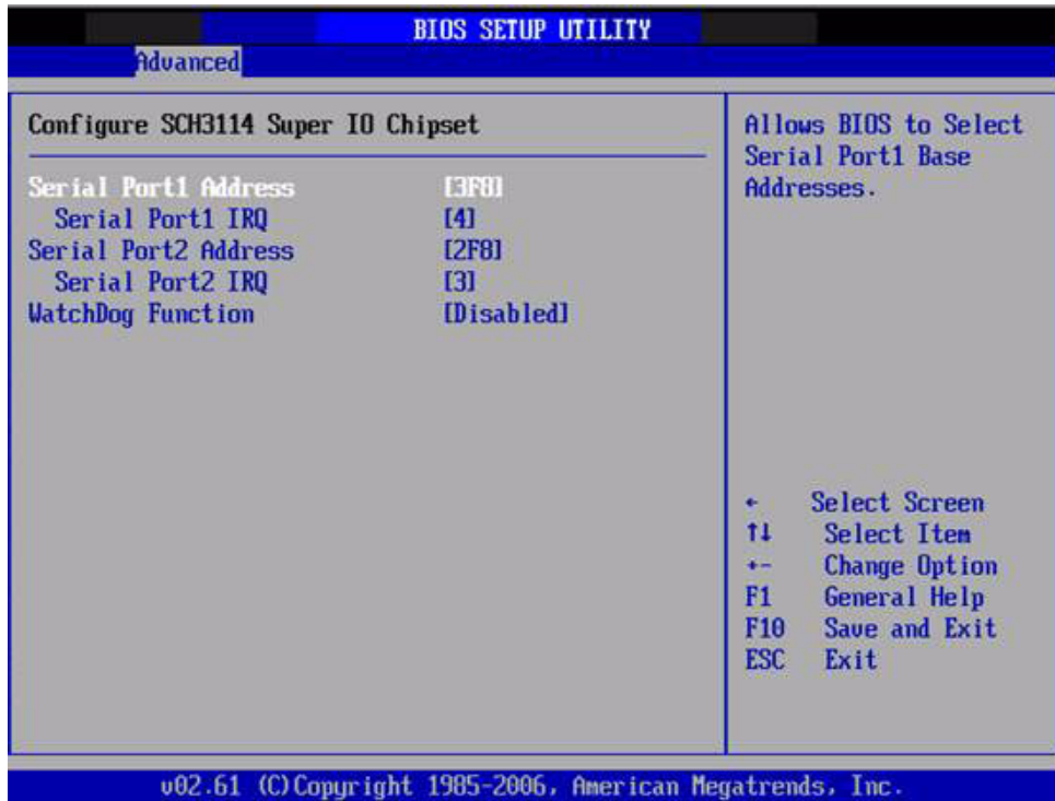
Figure 3.6 Super I/O Configuration
