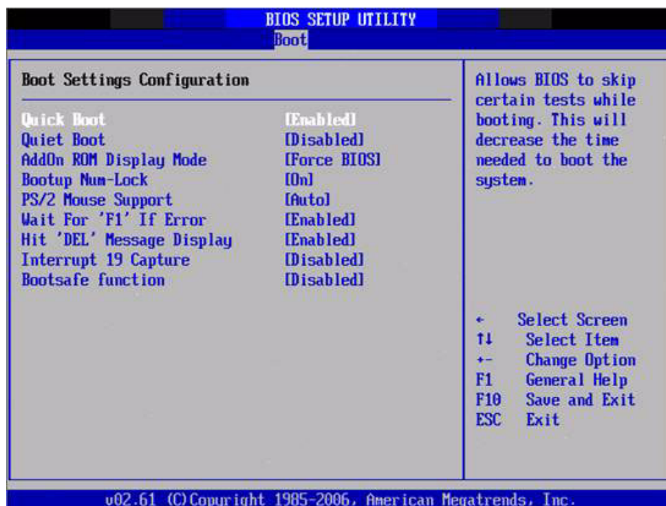
Figure 3.21 Boot Setting Configuration
