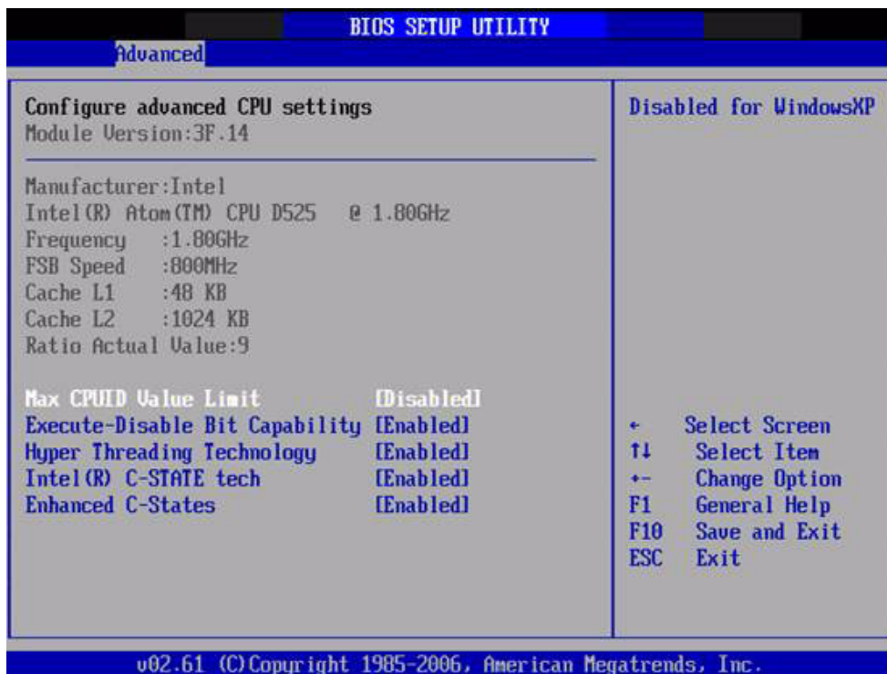
Figure 3.4 CPU Configuration Setting
