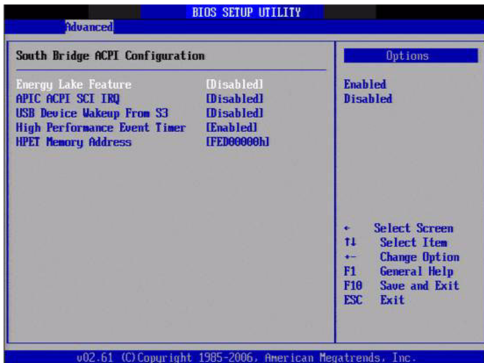
Figure 3.11 Chipset ACPI Configuration
