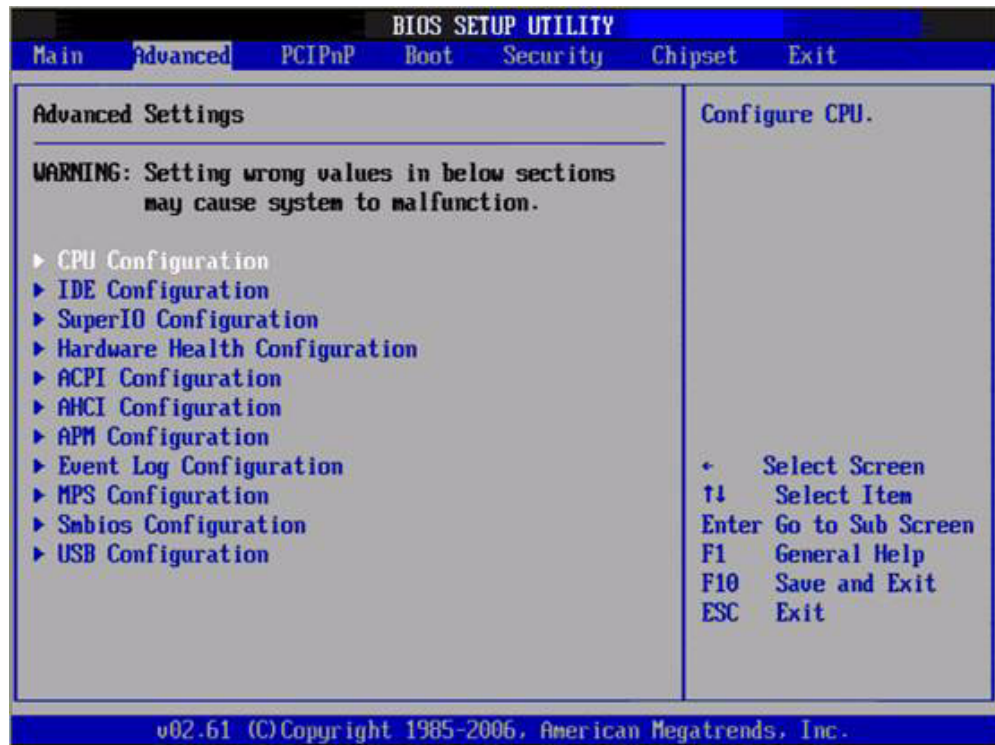
Figure 3.3 Advanced BIOS features setup screen
