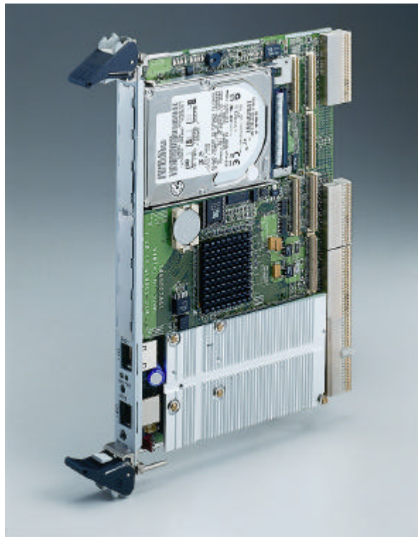
Figure 1-4: Complete assembly with heat sink, hard disk and a PMC module
