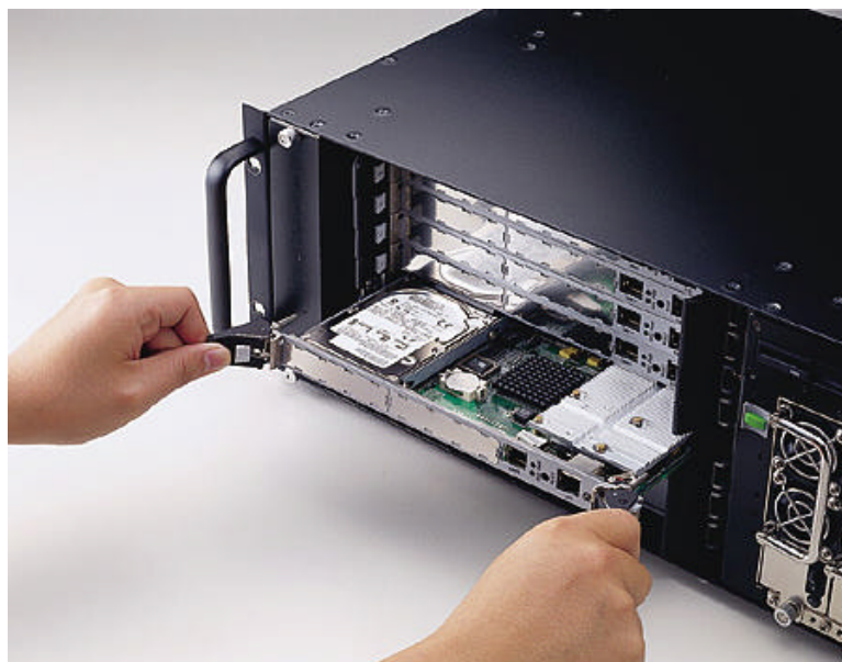
Figure 2-1: Installing the card into the chassis
