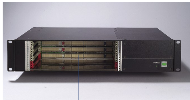
4-slot backplane with H.110 CT Bus
