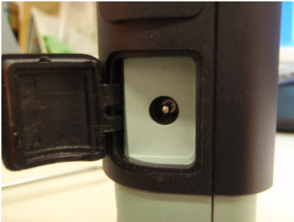
Figure3: Close the DC-in jack door on the MARS-3100 unit
