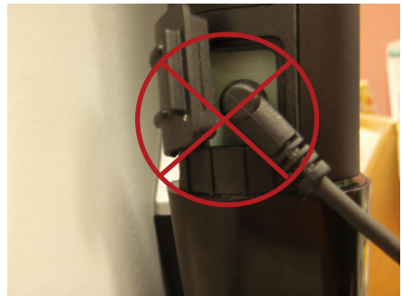
Figure1: Remove the adapter from MARS-3100 unit
