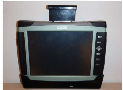
Figure 7: The MARS-3100 unit is sit on the cradle
