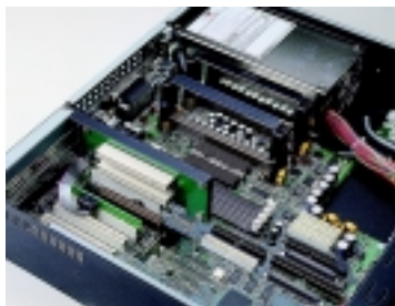
Integrated with Advantech's recommended motherboard, IPC-613 supports 2 PCI expansion slots.
