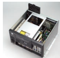
Solid disk drive housing & easy-to-maintain fan filter
