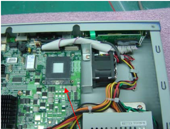
Unlock the socket of CPU as the symbol accordingly
