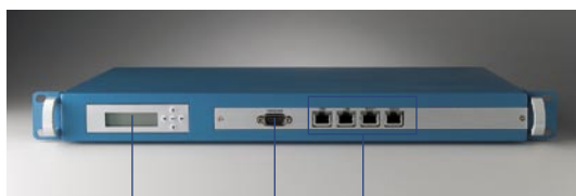
LCD display module RS-232 console port Four LAN ports
