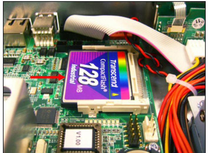
Figure 2-5: Install CF card
