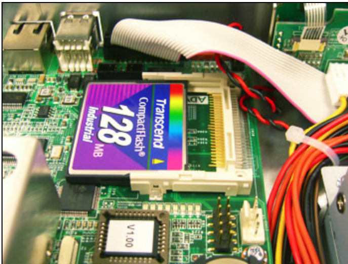
Figure 2-5: Install CF card
